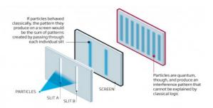
If observed, a single particle will pass through one of the two slits. If not observed, it passes through both.
